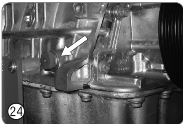
5.2.35. Remove VS5140.01 Crankshaft Locking Pin and refit crankshaft blanking plug, tighten to 30Nm. Remove the crankshaft pulley. Refit lower timing belt cover, the crankshaft pulley and the crankshaft pulley central bolt.
