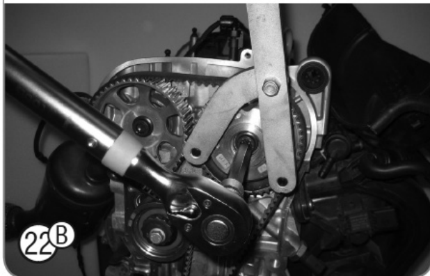
5.2.33. Using a suitable counter hold tool, such as VS783 Camshaft Holding Tool, tighten the central bolts of the camshaft sprockets to 50Nm+90°.
