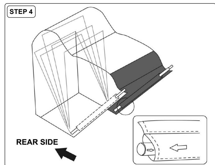
Fold the frame backwards, making sure the fabric covers the frame. Let the bottom unconnected tubes pass through the fabric sleeves.
