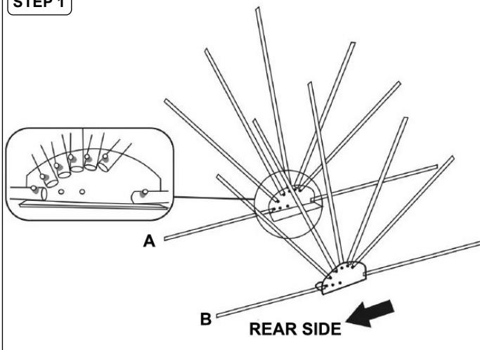
Position side frames (A) & (B) on the ground with the shortest tubes facing the front.
