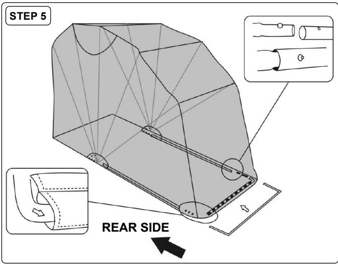
Pass the last angled bar (C) through the fabric sleeve and connect it to the side frames (A & B).
