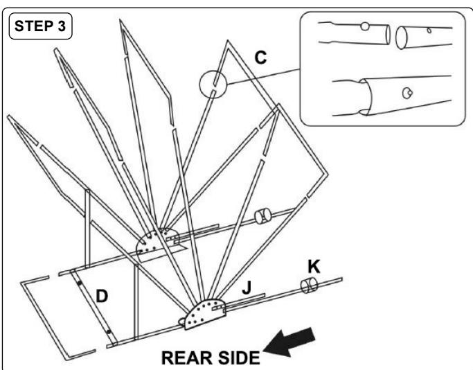
Connect angled bars (C) onto the side frames (A) & (B), leaving one angled bar (C) detached. Fix support bar (D) onto the side frames (A) & (B). Attach locking bar (J) onto the side frames (A) & (B) using the fixings provided. Slide rings (K) onto the frame. Leave in the unlocked position shown when assembling the shelter.
