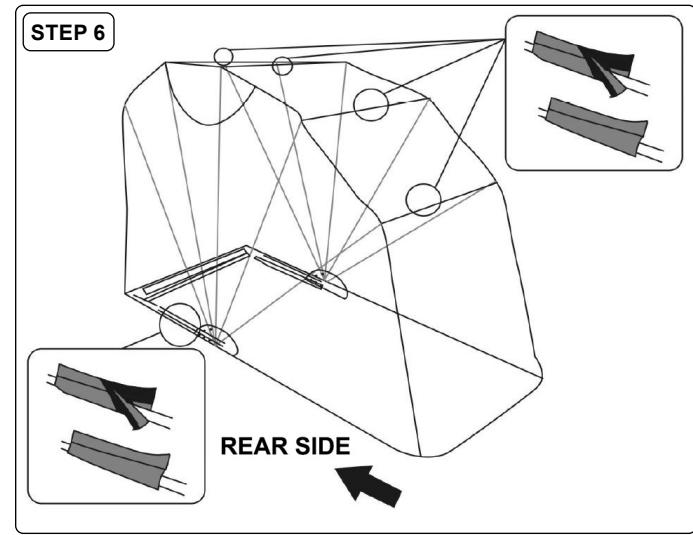
Wrap the frame with the velcro sewed on the fabric cover at the locations shown.
