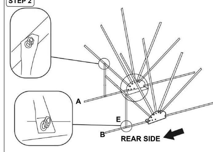
Attach supports (E) onto the side frames (A) & (B), using the fixings provided.
