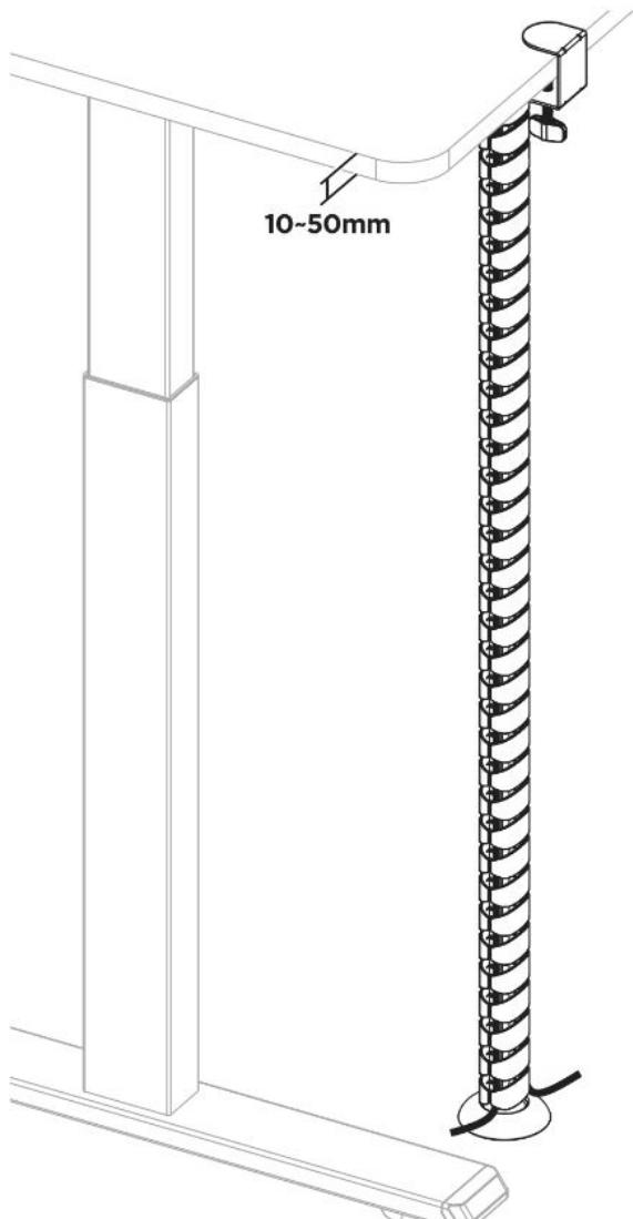
**Note:** When joining the spine parts, ensure the same channels on the same side.
