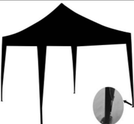
Raise or level the shelter using adjustment holes found near bottom of each outer leg. Secure with guide ropes/weight bags.
